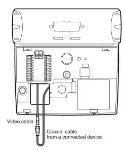
4. Connect the cables to the Wiegand and alarm output connectors as shown in the illustration. (Refer to p. 14 for details on each cable connection.)
